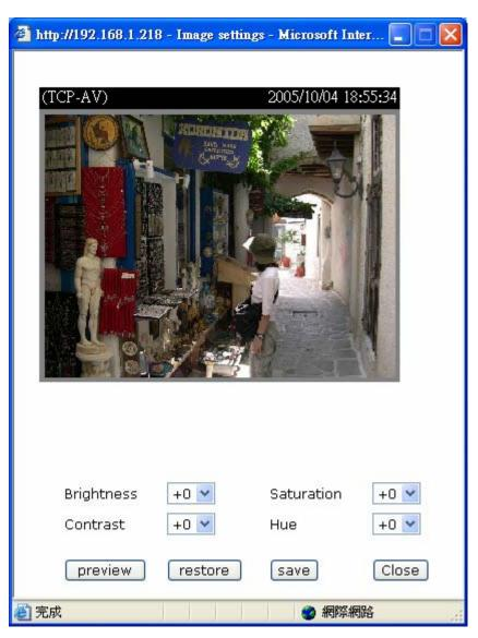
"Contrast", "Hue" and "Saturation" for video compensation. Each field has eleven levels ranged +5. In from -5 to "Brightness" and "Contrast" fields the value 0 indicates auto tuning. The user may Preview press to fine-tune the image. When the image is O.K., press save to set the image settings. Restore Click on this to recall the original settings without incorporating the changes.
